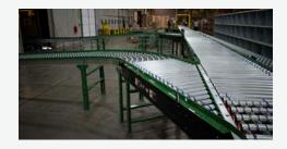
Installed 24V MDR technology with 36" accumulation zones. The infeed conveyor feeds 3 separate lines.
