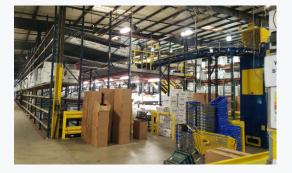
After an assessment of the data provided by the client, PeakLogix introduced a 2-Level Pick Module which uses bar code scanning and conveyor to intelligently route cartons into the required storage zones for picking. The conveyor is lined with carton flow on each side, providing 3 levels of storage.
