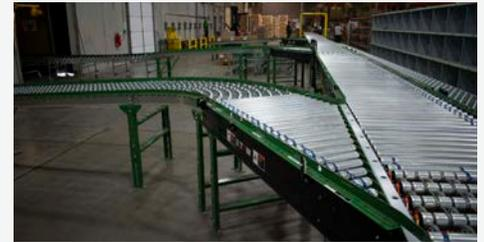
Installed 24V MDR technology with 36" accumulation zones. The infeed conveyor feeds 3 separate lines.
